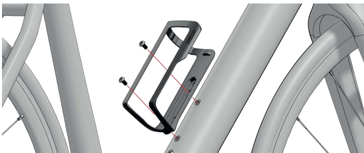
Figure 3-12 BIKEDRIVE AIR | Mounting Ranger Extender bracket
